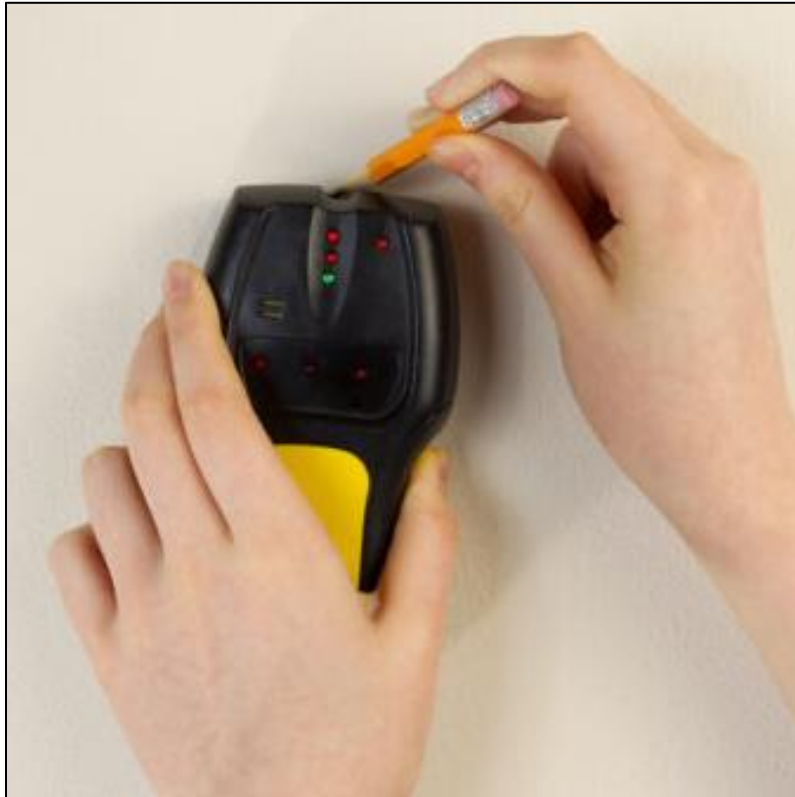
Figure 4.6 - Handheld Stud Finder Use Concept Example [23]
