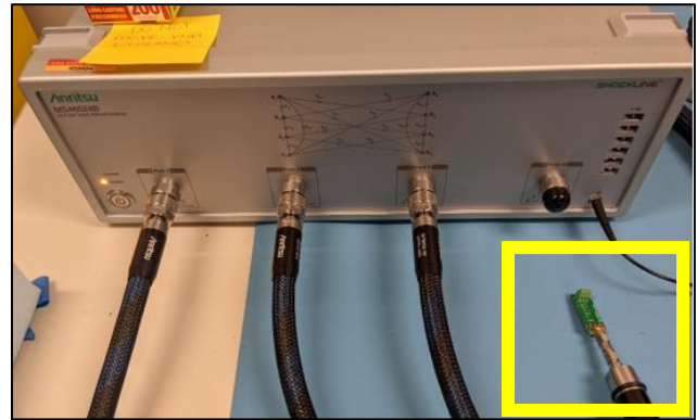
Figure 4.15 – Picture of Physical Test Board/VNA Measurement Process (Test Board Emphasized by Yellow Box)
